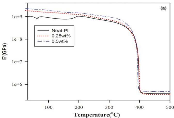
Figure 3: Elastic Modulus vs. Temperature
